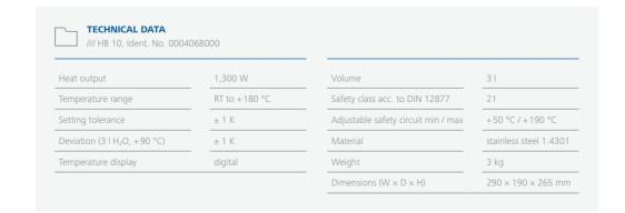
HB 10 HEATING BATH: FOR A LOW VOLUME AND FAST HEAT-UP TIME
