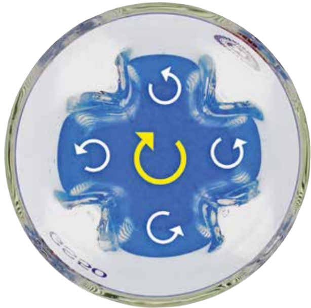
GS vessel principle (viewed from top)
